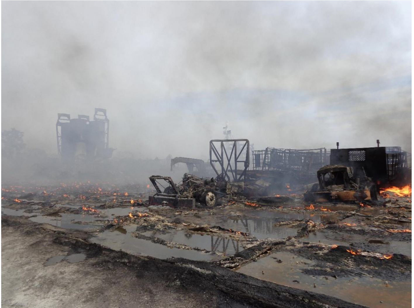
Figure 3 shows an example of a spill of fracking fluids. The photo is from the U.S. Environmental Protection Agency and shows a fire on June 28-29, 2014 at the Eisenbarth Well operated by Statoil (since renamed Equinor) in Monroe County, Ohio. The photographer is not listed. 74 According to an EPA report, trade secret fracking chemicals along with other chemicals were spilled because of the fire. Fluids that may have contained the trade secret chemicals ran off the well pad into a tributary of the Ohio River. An estimated 70,000 fish died. 75
